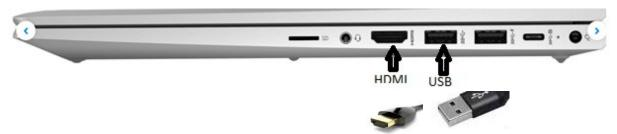
These two cables are needed to share your laptop screen with that of the ProWise board and to use the touchscreen functionality of the screen.
